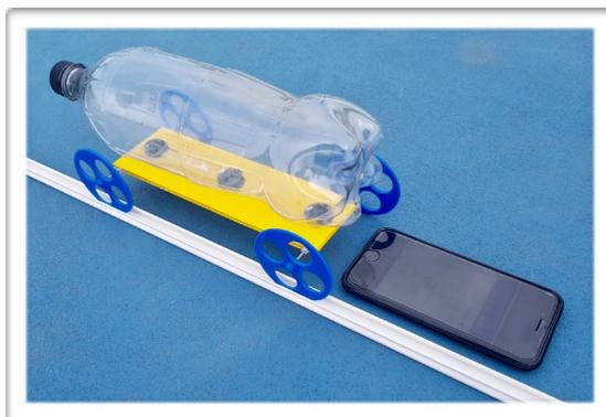
In this measurement we use the **light sensor** of the mobile phone and a light source (lamp or sunlight). Simply start the light intensity recording on the phone and place the phone **face-up** next to the car track. OneCar has enough clearance to move over the phone while the phone is recording the light levels. The resultant graph on your phone should be similar to this:
